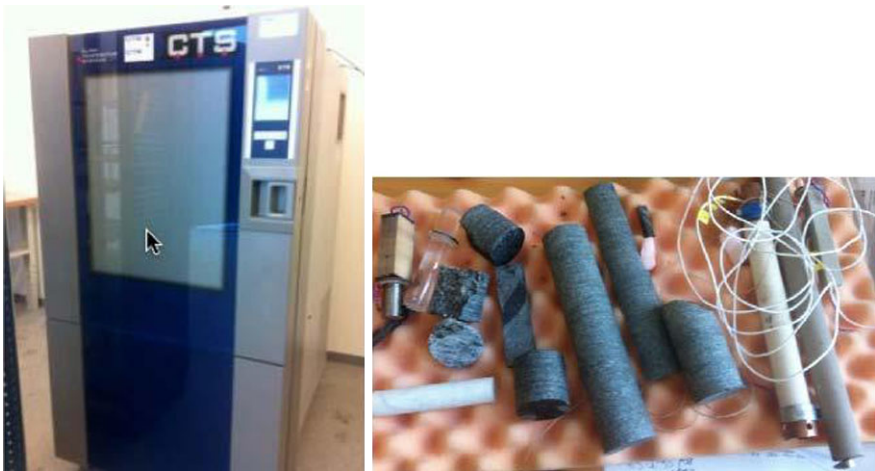
Fig. 2 Left: The climate chamber. Right: A few different rocks and a couple of other test samples
