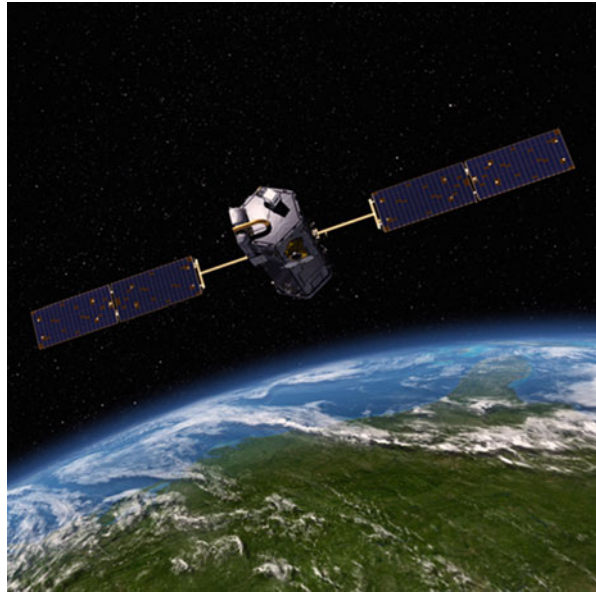
Fig. 3.10 The Orbiting Carbon Observatory-2, scheduled for launch in 2015, will perform precise, time-dependent measurement of atmospheric CO 2 levels. (Artist rendition of the OCS-2 by John Howard, JPL: http://oco.jpl.nasa.gov/ , open source)
