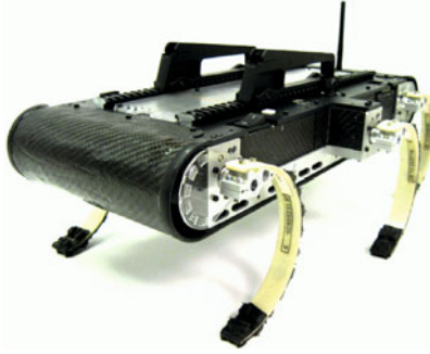
Fig. 1 A specimen of the RHex family of legged robots, designed in University of Pennsylvania. Reproduced with permission from [4]
