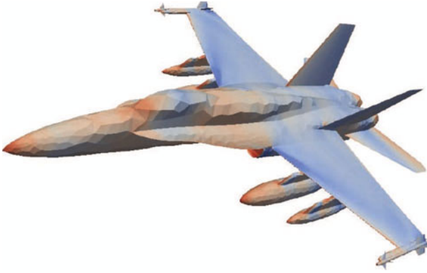
Fig. 8.5. F18/A configuration at M_\infty = 0.99 : steady-state surface pressure
