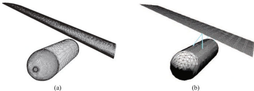
Fig. 8.1. High-dimensional aeroelastic model of a wing-store configuration. (a) CFD surface grid; (b) Finite element structural model
