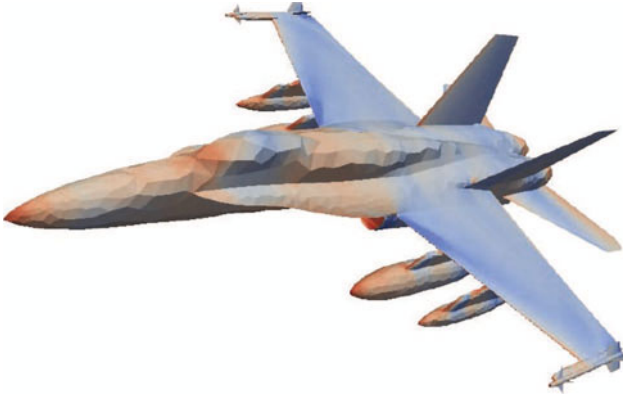
Fig. 8.5. F18/A configuration at M_\infty = 0.99 : steady-state surface pressure
