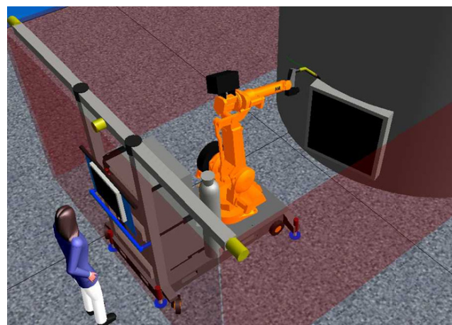
Figure 5. Concept of a freely transferable robot platform used in a process application.
