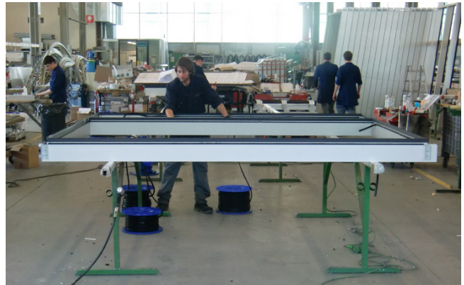
Figure 2: Industrialized preassembly line of façade modules.
