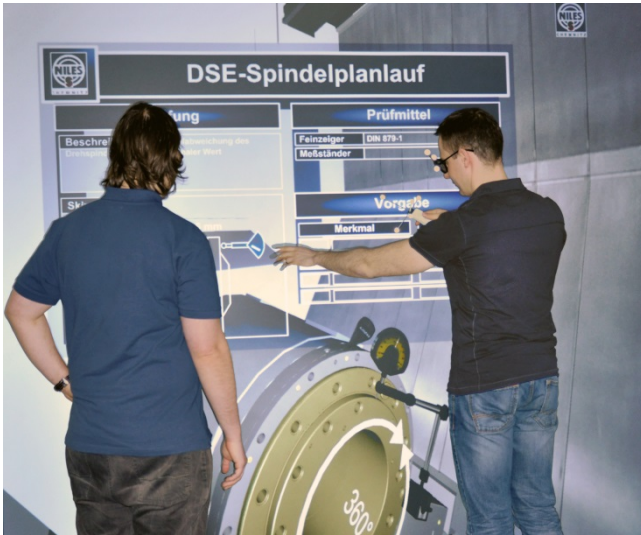
Figure 2: Example of an Immersive Presentation for measuring the concentricity of a spindle in a VR training application in the field of maintenance.
