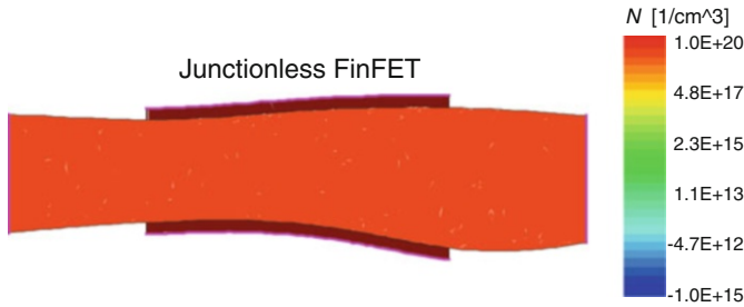
Fig. 7.19 Representative 32nm JL-FinFET with 1nm LER applied to the fin edges
