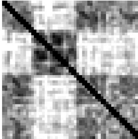
Fig. 1. The similarity matrix of a recording containing two speaker change points
