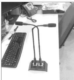
Fig. 1. The symmetrical two microphone system
