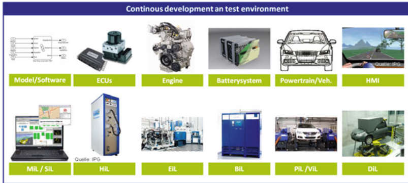
Fig. 4 The X-in-the-loop-process in AVL InMotion/IPG CarMaker: model- ( MiL ), software- ( SiL ), hardware- ( HiL ), engine- ( EiL ), battery- ( BiL ), powertrain- ( PiL ), vehicle- ( ViL ) and driver-in-the-loop ( DiL )
