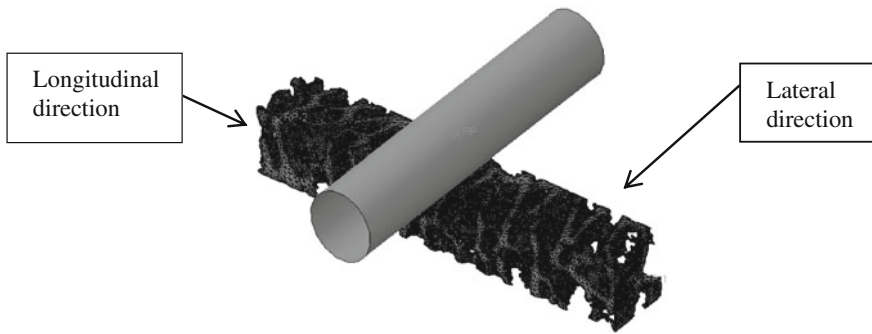
Fig. 3 Epiphysis model with rigid cylinder assembled
