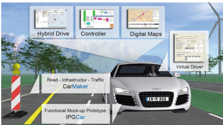
Fig. 3 Virtual test drive in AVL InMotion/IPG CarMaker (source IPG Automotive)
