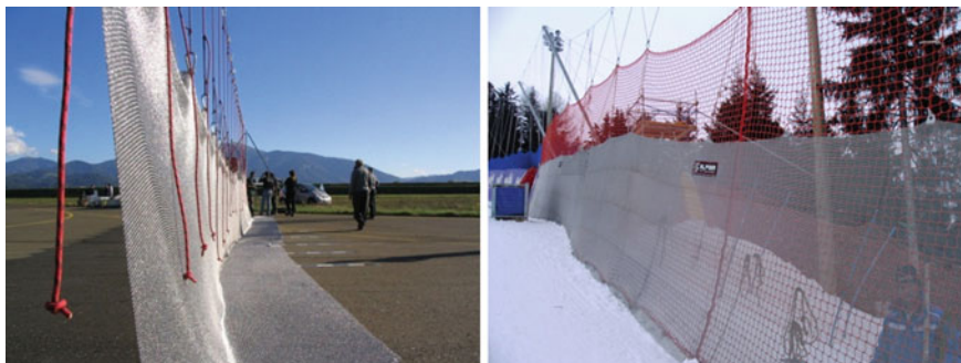
Fig. 3 Impact configurations: test situation ( left ); mesh application on site ( right )
