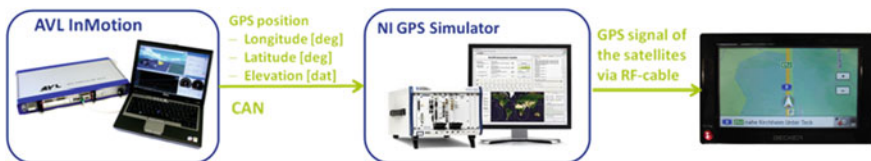
Fig. 6 Structure of the demonstrator consisting of the AVL InMotion real time PC, the NI GPS simulator and a mobile navigation system
