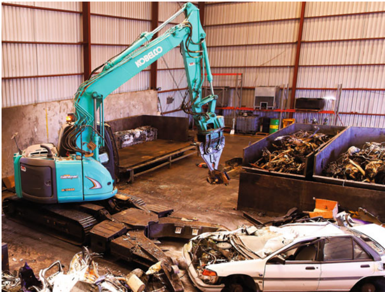
Fig. 1 An excavator-based multi-dismantling machine
