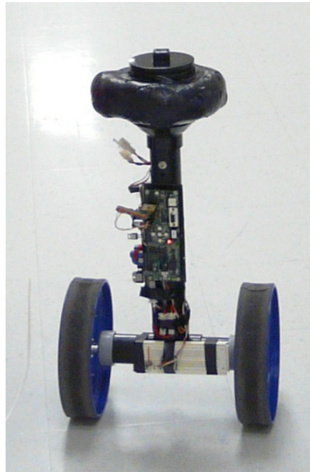
Fig. 1. InPeRo, an inverted pendulum robot, Courtesy of É.T.S
