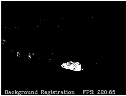
Fig. 2. Results returned by the frame difference with background registration method
