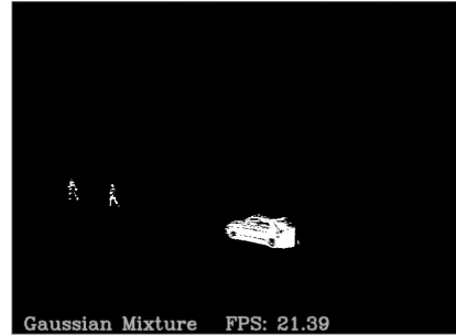
Fig. 5. Results returned by varying Gaussian distributions number method
