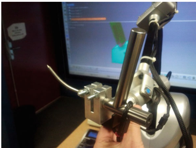
Fig. 13.3 The instrument tightened by the piece is tied to the haptic arm
