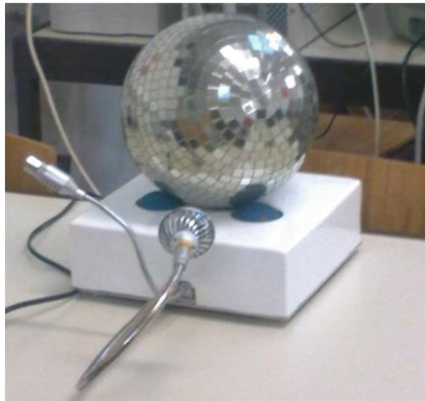
Fig. 21.1 Sketch model of the optokinetic simulator developed
