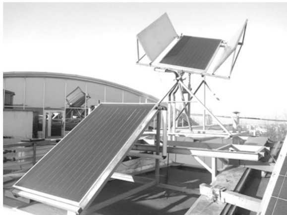
Fig. 15 Solar tracking system with low concentration for solar thermal collectors, patent request no. A/00109/2012
