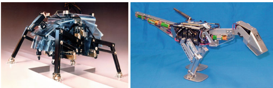
Fig. 5 Examples of leg mechanisms in walking robots
