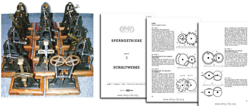
Fig. 2 Physical demonstration models from the University of Hannover ( left ) and figures and descriptive texts in books ( right ) as examples for content sources for mechanism descriptions
