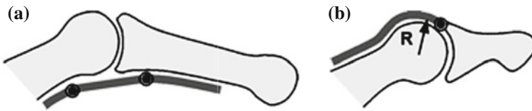
Fig. 5.8 Models for the tendons crossing the joints: (a) Straight lines, (b) Landsmeer's model I
