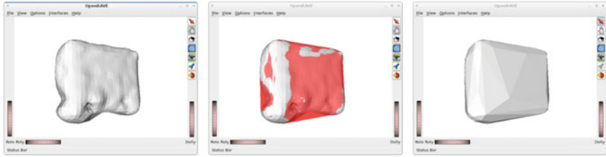
Fig. 4.15 Example of convex hull decomposition of the generated triangular mesh
