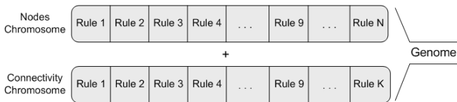
Fig. 1. This is how the genome looks like with the genome split into two chromosomes . The first chromosome is responsible for generating the cells/nodes whereas the second chromosome is responsible for generating the connectivity of the network.
