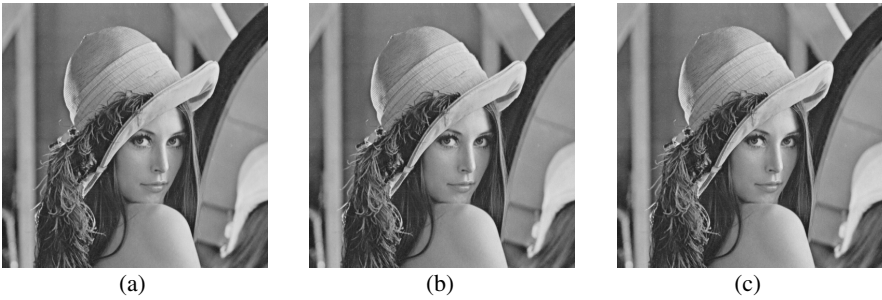
Fig. 2. Stego-images of 'Lena'. (a) Payload=400,000 bits, PSNR = 51.14 dB. (b) Payload=650,000 bits, PSNR = 48.31 dB. (c) Payload=1,000,000 bits, PSNR = 43.12 dB.
