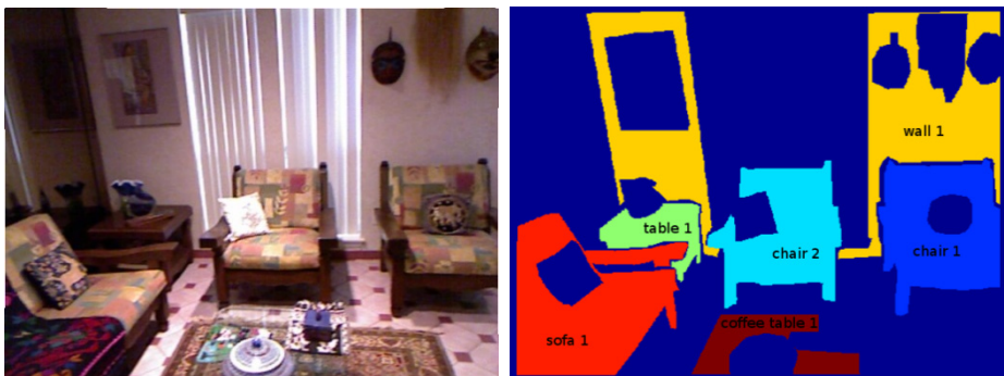
Fig. 3. This figure shows an example room with segmented spatial structures such as pieces of furniture and walls
