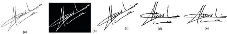
Fig. 1 Results of preprocessing on an signature sample image from GPDS-100 dataset (a) Input signature image (b) Binarized (c) Noised removed image (d) Rotated by an angle of 29.101 degree and thinned image (e) Normalised image
