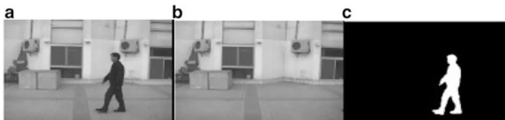
Fig. 59.1 Examples of moving silhouette extraction: (a) An original image, (b) the background image constructed by three-frame difference method, (c) the extracted silhouette form
