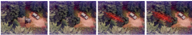
Fig. 78.2 The original image is shown in the first column; the tampered image is pictured in the second column; the detection results using SIFT and new algorithm are reported in the third and fourth column, respectively
