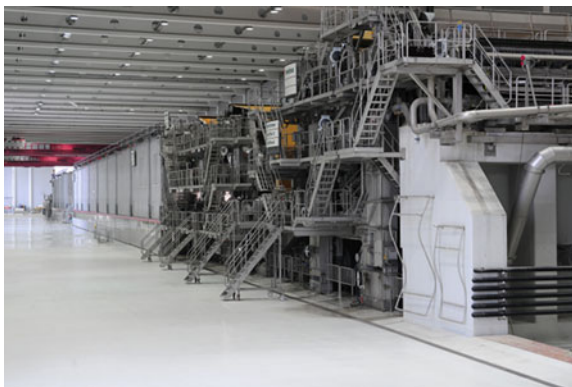
Fig. 1.1 The dimensions of a paper machine. The height of the machine is approximately 8 m, the width 12 m and the length 120 m. Open draws are mainly hidden inside the drying section, located center left in the photo. (Photo courtesy of Metso Paper)
