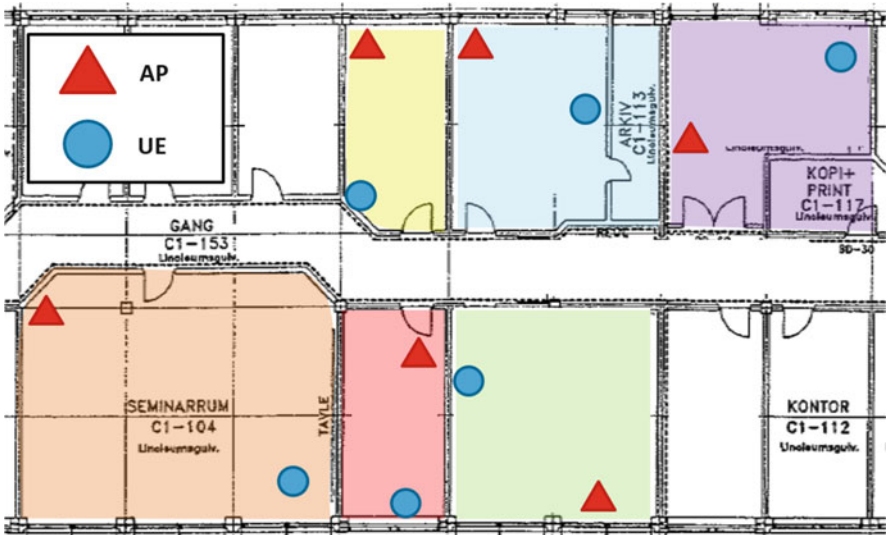
Fig. 12.12 Deployment of nodes of the ACCS test bed across office premises at Aalborg University
