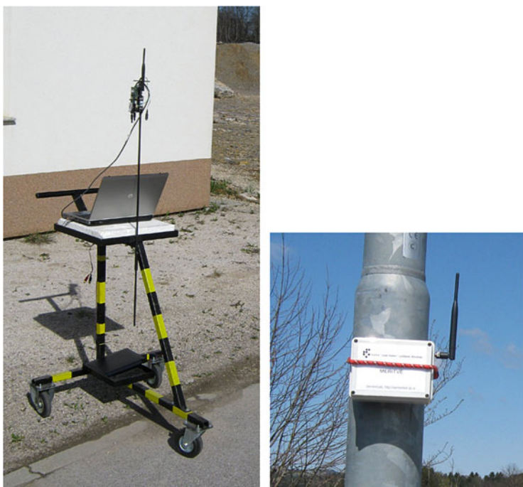
Fig. 13.13 VESNA node (T/R) with a PC on a mobile measurement platform (left) and VESNA node (E) at a fixed location (right)
