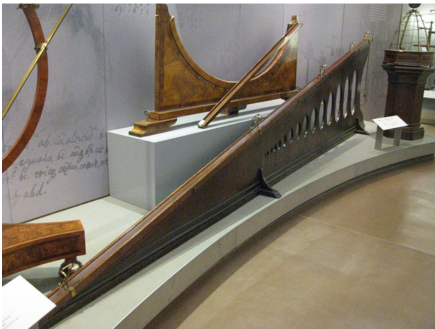
Fig. 7.20 Galileo's inclined plane (note the bells placed at intervals for the purpose of measuring the acceleration of balls), Galileo Museum, Florence
