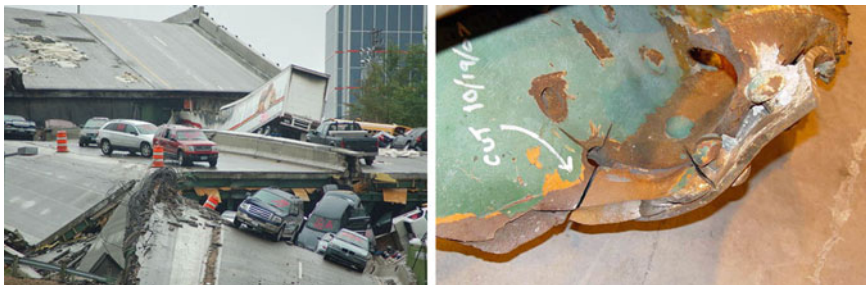
Fig. 13.31 Photo on left of the Minneapolis bridge collapse; photo on right showing fracture in gusset plate
