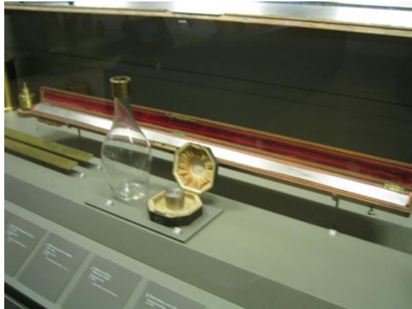
Fig. 8.22 Photo of platinum bar representing the meter in the Musée des Artes et Metiers, Paris
