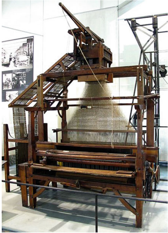
Fig. 8.17 Photograph of a Jacquard loom
