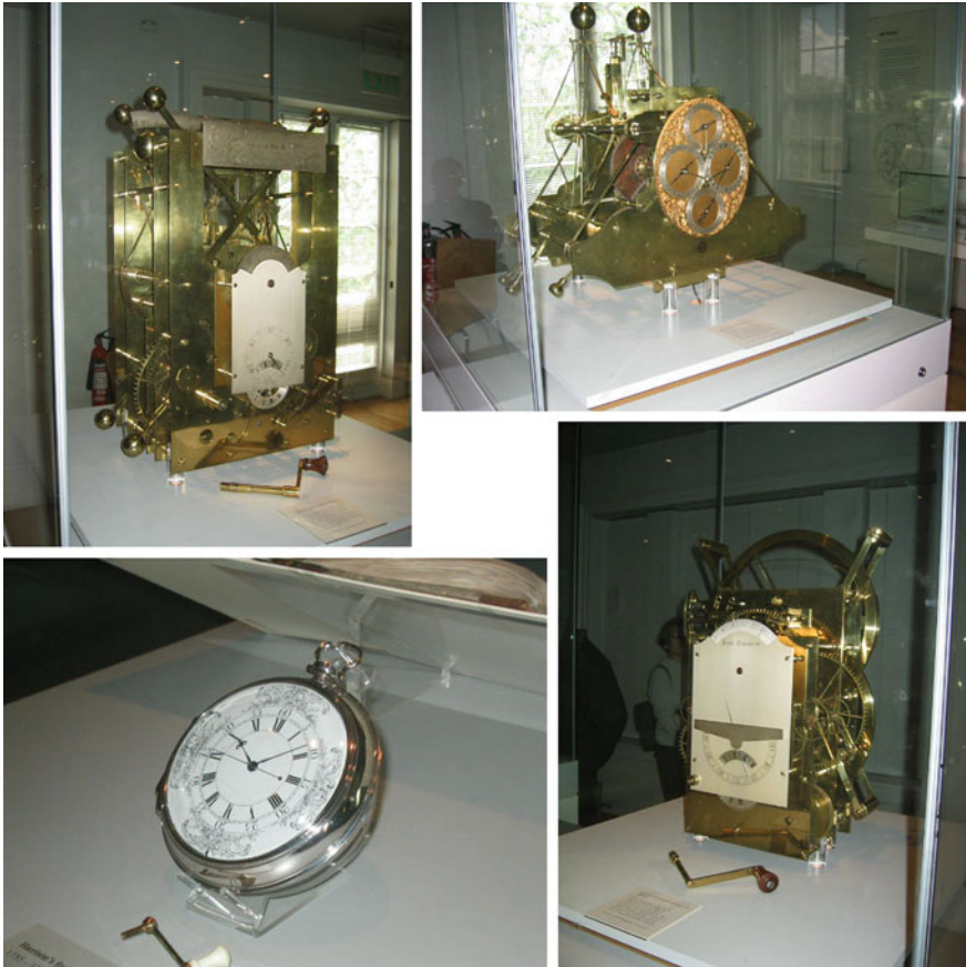
Fig. 8.21 Photos of John Harrison's chronometers, numbers one through four clockwise from top left
