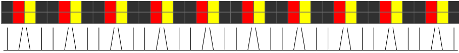
Fig. 3. Excitation waves travelling in a 40 \times 2 cylindrical lattice. The ‘equivalent’ cilia metachronal wave is depicted below the CA states (grey is excited, white is refractory and black is resting).
