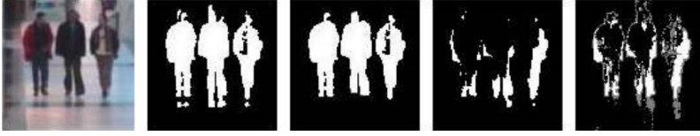
Fig. 3. Comparison - from left - 1. Original picture, 2. Original eigenbackground, 3. Eigenbackground 16 \times 16 frames, 5. MOG, 6. MOG2
