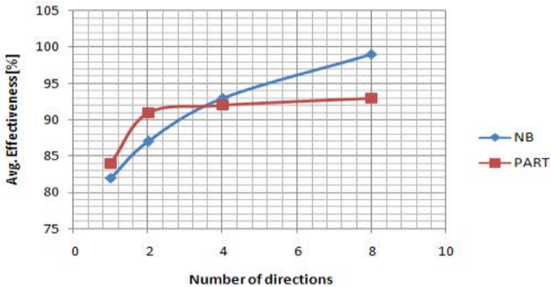
Fig. 4. The average effectiveness of two methods of classification (PART and Naive-Bayes - NB) for the varying number of directions that a simple cell is sensitive to
