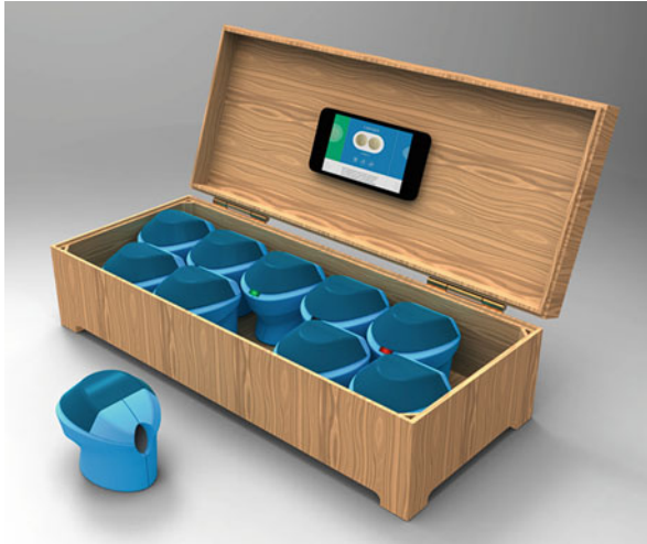
Fig. 6 The iRxReminder iLidRx™ medicine cabinet is a system designed to integrate into a home setting to support complex medication schedules. The system is managed from a cloud-based control center, and each pill-dispensing device holds a single medication. The devices communicate via Bluetooth LE when medication is dispensed. If the medication is not dispensed on time, the system sends the app on the smartphone an alert. The alert can also be directed to any display in the home (e.g., television display), and an alert from the voice interface could also alert the person (e.g., Amazon Echo)
