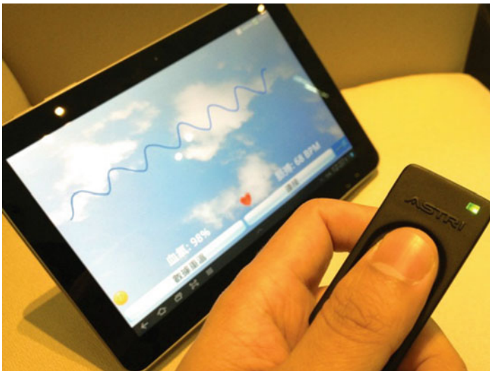
Fig. 13 E-health system is used to measure elders' blood pressure, blood pulse and blood oxygen level
