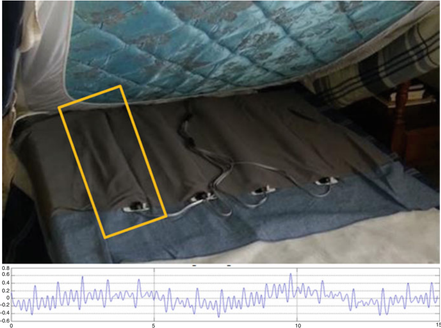
Fig. 6 The University of Missouri hydraulic bed sensor installed under the mattress with four transducers. The graph shows the combination of respiration and ballistocardiogram signals that are captured using this sensor
