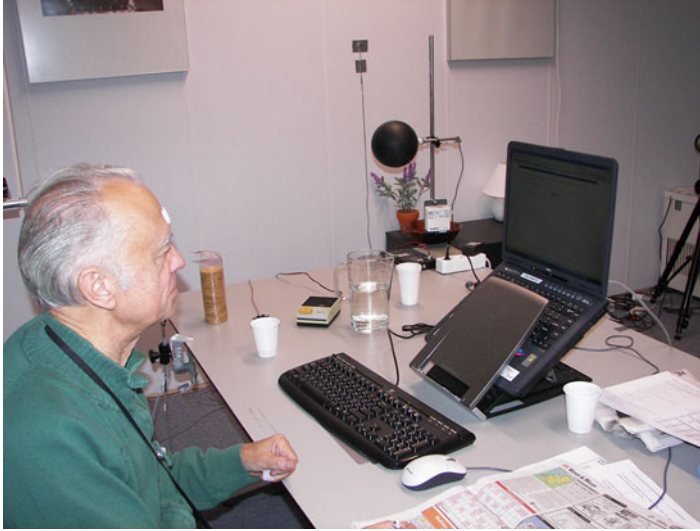
Fig. 2 Older subject in climate chamber in order to study the differences in thermal comfort between young and older adults (Schellen et al. 2010)
