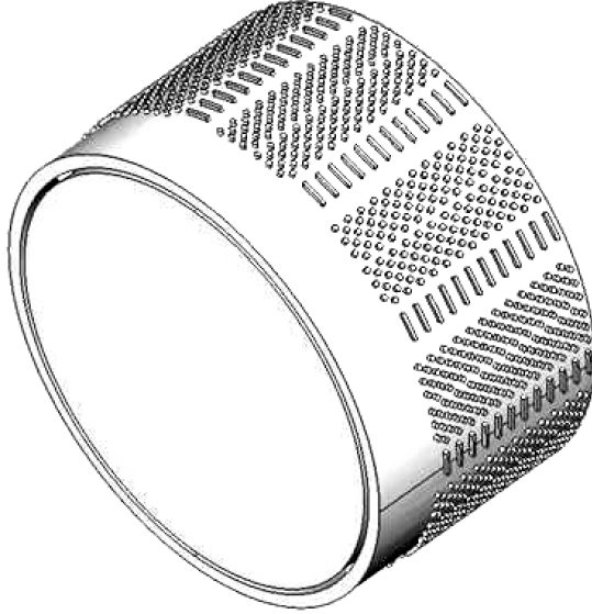
Fig. 3. Burner mantle CAD model
