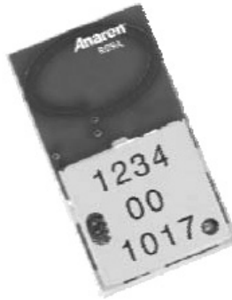
Fig. 18.5. An example radio transceiver module A1101R09A from Anaren incorporates TI CC1101 transceiver chip, size 9x16x2.5 mm. (Source anaren.com )
