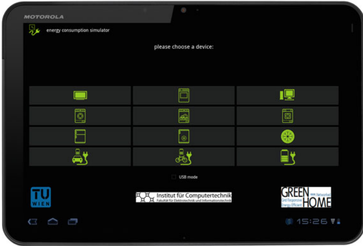
Fig. 10.2 A screenshot of the energy consumption simulator’s main menu that shows all devices that can be simulated (TV set, washing machine, refrigerator, rechargers, etc.). Each simulation runs in real time, therefore real time values are sent to the Gateway using ONENET via an attached communication node. If the simulator is not connected to a real network of devices, it offers a much faster simulation mode, too, in order to easily see consequences of events
