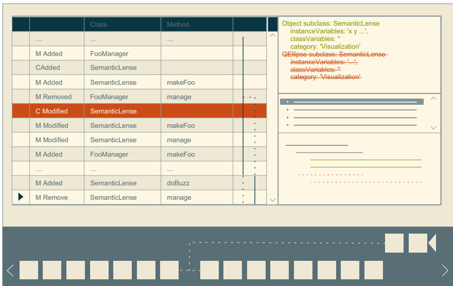
Fig. 6 The version browser provides a tabular view on change history. Selecting a row shows corresponding diff information in the panes to the right
