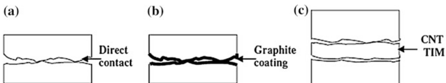
Fig. 7.13 Schematic of contacting surfaces: a in direct contact; b separated by graphite coating; c separated thin sheet of CNT interface material (Shaikh et al. 2007. Reprinted by permission from Pergamon Publishers)
