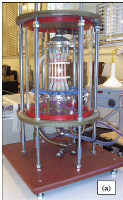
Fig. 8.6 a View of the experimental apparatus with the test section in place. b The test section with seven tubes and a fin sheet (Cheng 2006)
