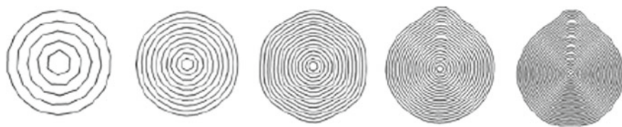
Fig. 13 Cross-sectional views of relaxed MWNTs indexed by (2,8)/(4,16)/\dots/(2n,8n) . The wall numbers n are 5, 10, 15, 20, and 25 from left to right , and all the MWNTs are 20 nm long. After Ref. Huang et al. (2011)
