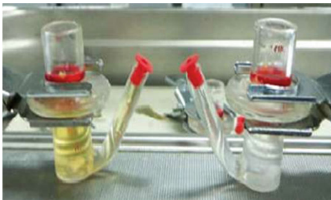
Fig. 1.7 Image obtained in our laboratory after a test of skin integrity with a marker (Balaguer et al. 2006) on a diffusion cell which proved to be discarded ( left ) and one that proved to be valid ( right ) after the corresponding analytical determinations of the marker in the receptor fluid
