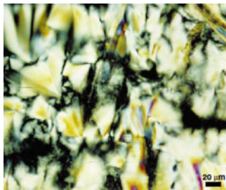
Fig. 2 Fan-like texture of monodisperse PBLG in \text{CHCl}_3 :TFA mixture. Reproduced from [14] with permission of the publisher
