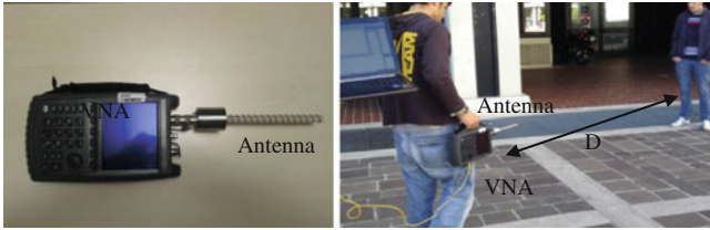
Fig. 2 Photo of the electromagnetic obstacle detection sensor. The EM portable system ( left ); The system in use ( right )
