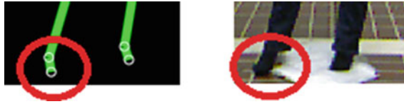
Fig. 5 Detail of feet joints location by Kinect, dummy case
