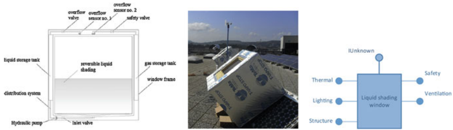
Fig. 2 Functional schema of the reversible liquid shading window ( left ), the two test cells during the outdoor experimental campaign ( center ) and the component model ( right )
