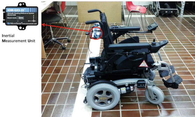
Fig. 1 The smart electric-powered wheelchair with the IMU sensor
