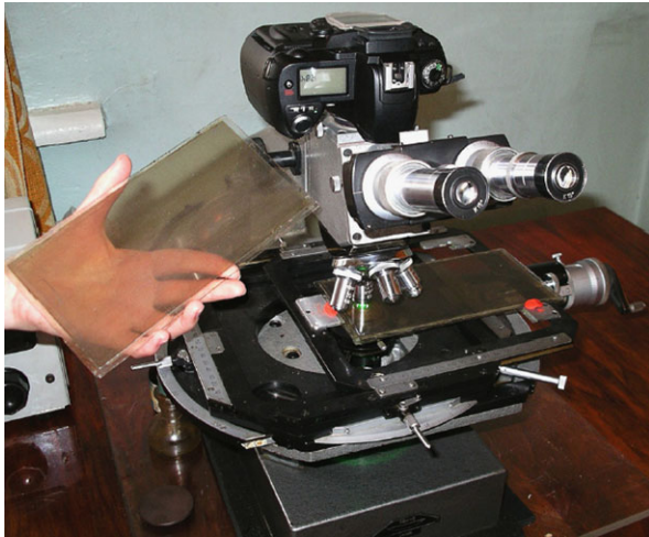
Fig. 3.5 Photograph of an NTE pellicle on a glass substrate and of a microscope with an installed photo camera
