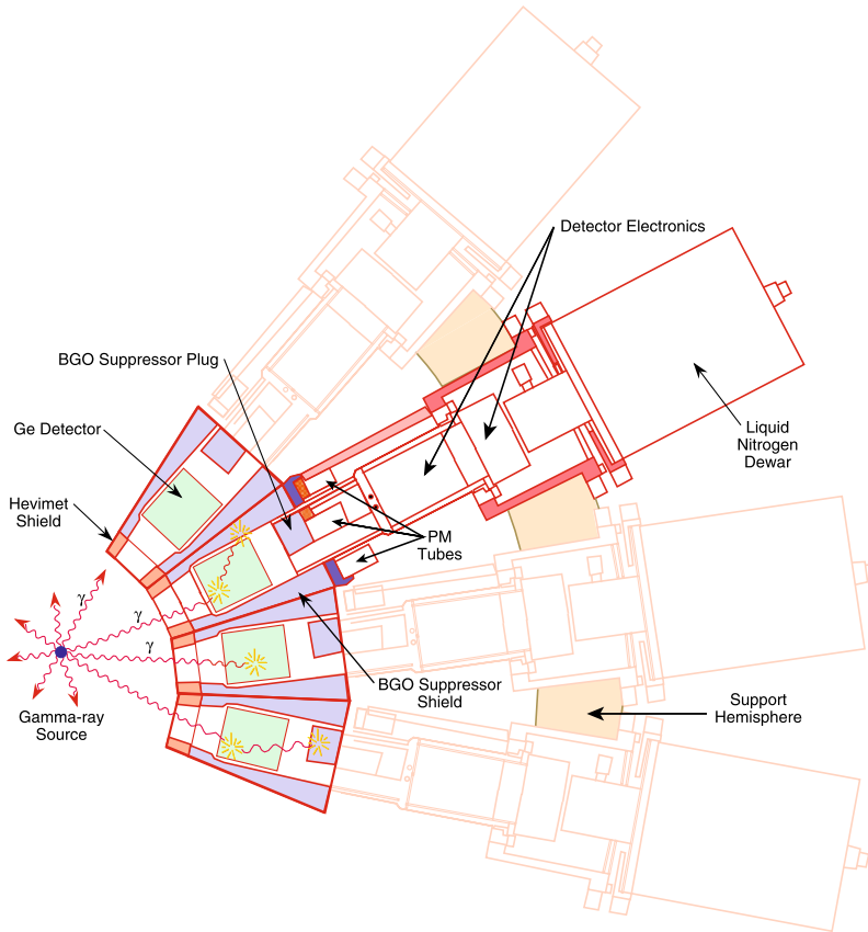
Fig. 2.8 Schematic of a Gammasphere detector module
