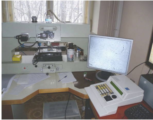
Fig. 3.27 Automated microscope PAVICOM-2 (FIAN, Moscow)
