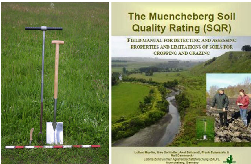
Fig. 2 Essentials for the fieldwork of soil rating. The spade is used for digging the pit and for the spade test of soil structure analysis. The knife is used for checking soil strength and coherence of aggregates. The auger is important for identifying soil texture and other properties like a shallow watertable from 1 to 1.5 m depth. The field manual contains all rating tables. In order to assess the drought risk, monthly data of precipitation and potential evapotranspiration are required. Data can be taken from the local climate estimator New_LocClim 1.10 (FAO 2006b) before starting fieldwork
