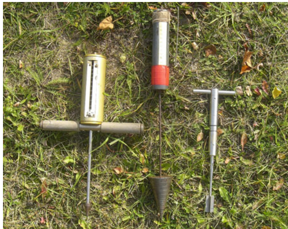
Fig. 1 Devices for measuring soil strength. a Penetrometer. b Sink cone. c Vane shear tester
