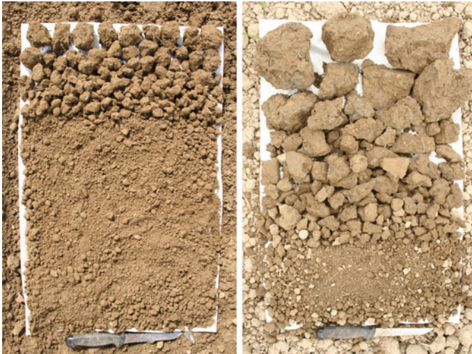
Fig. 11 Different features of soil aggregates in New Zealand (Structure indicators of the VSA drop-shatter procedure of Shepherd 2000). On the left is Manawatu silt loam Haplic Fluvisol (Eutric, Siltic, Drainic) with moderately good structure, rating of 1.5 (0 = worst, 2 = best) and on the right is Kairanga clay Fluvic Gleysol (Eutric, Clayic, Drainic) with poor structure, rating of 0
