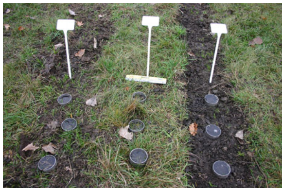
Fig. 5 Water infiltration on cattle trampling pathways as compared with adjacent parts of the paddock
