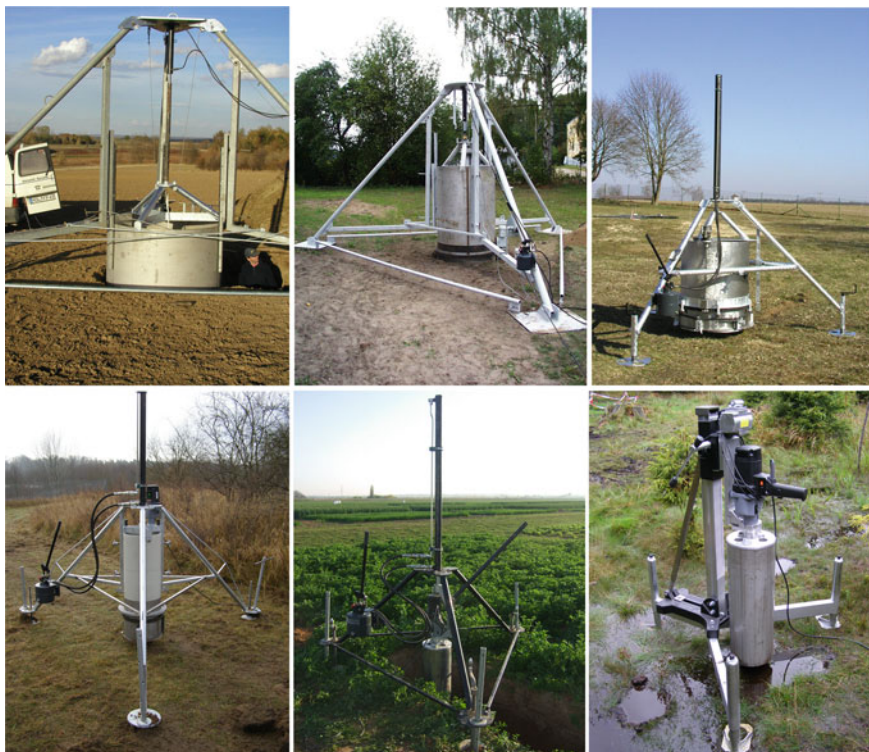
Fig. 2 Types of cutting tool available for obtaining undisturbed soil monoliths of different sizes and from various sites (starting from top left —surface area of: 2, 1, 0.5, 0.07, 0.03 and 0.03 m 2 for peat soil)
