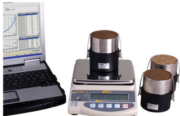
Fig. 6 Sample is clamped, placed on a balance and connected to a computer
