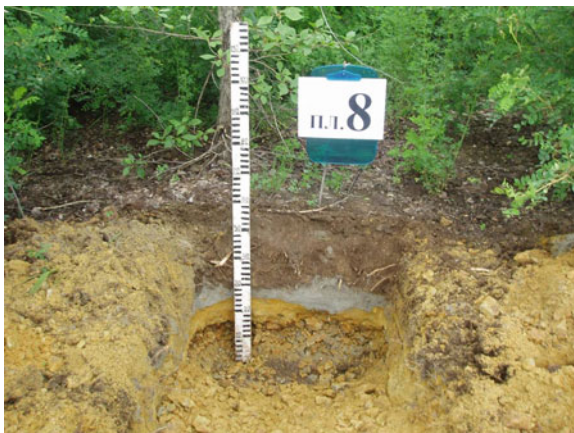
Fig. 1 Pit. Artificial profile made of Loam + technical sand + dump—site 8
