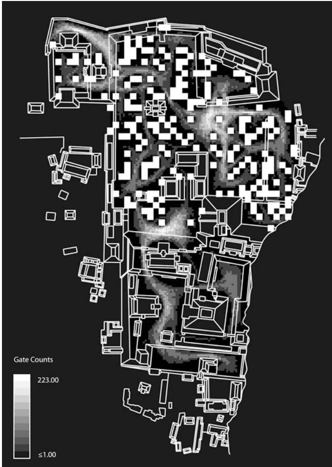
Fig. 7 Agent simulation at Copan. Note great Plaza with 20 % random distribution of obstacles
