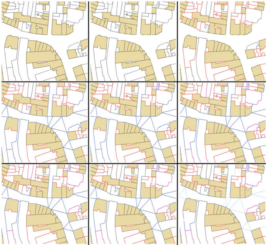
Fig. 7 Example of the BLT identification process in nine stages on the basis of the Winchester's MasterMap outline base plan ( black ). From left to right, in order of the BLT identification added: Type 1 ( brown ); Type 2 ( light green ); Type 3 ( red ); Type 5 ( blue ); Type 8 ( purple ); Type 9 ( pink ); Type 4 ( dark green ); Type 11 and 12 ( grey ); virtual boundaries ( clear blue ). For visual clarity Type 1 has been converted into filled polygons. Note how the triangles of road segments are exclusively virtually bounded. (Based upon Ordnance Survey mapping. © Crown Copyright 2013. All rights reserved. An Ordnance Survey (EDINA) supplied service.)
