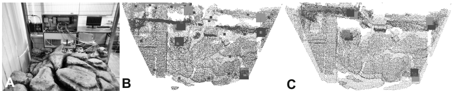
Fig. 1 Terrain mockup (A), point clouds with NARFs prior to matching (B), matching result NARF+ICP (C)
