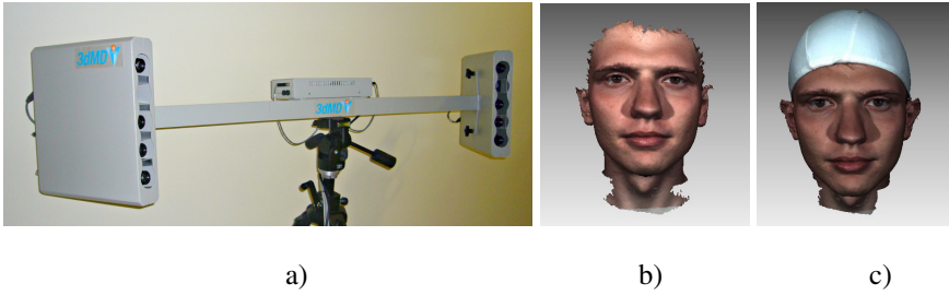
Fig. 1 3dMDFace scanning system: a) measurement device, b) single mesh from scanner, c) reconstructed mesh model of head
