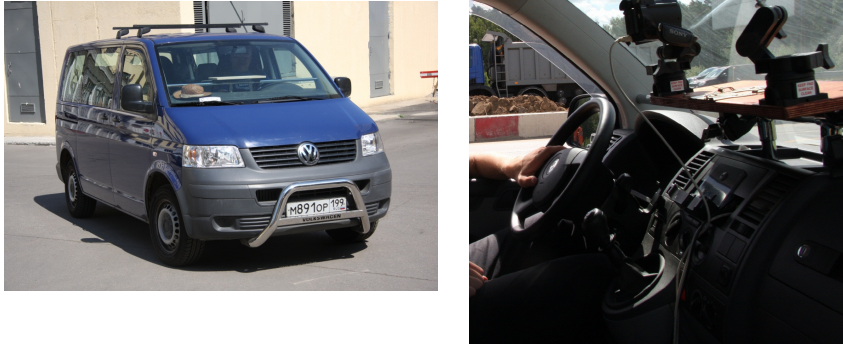
Fig. 1 Mobile laboratory on the basis of the Volkswagen Transporter (Property of MADI)
