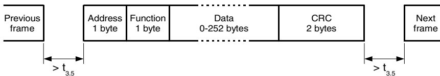
Fig. 1 Modbus RTU frame; t_{3.5} is the minimum time separating adjacent frames
