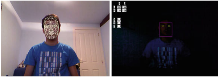
Fig. 2 Face and eye tracking based on Kinect sensor, left to right, CANDIDE-3 face model in Kinect Face Tracking Demo [12], face and eye tracking under poor illumination [13]
