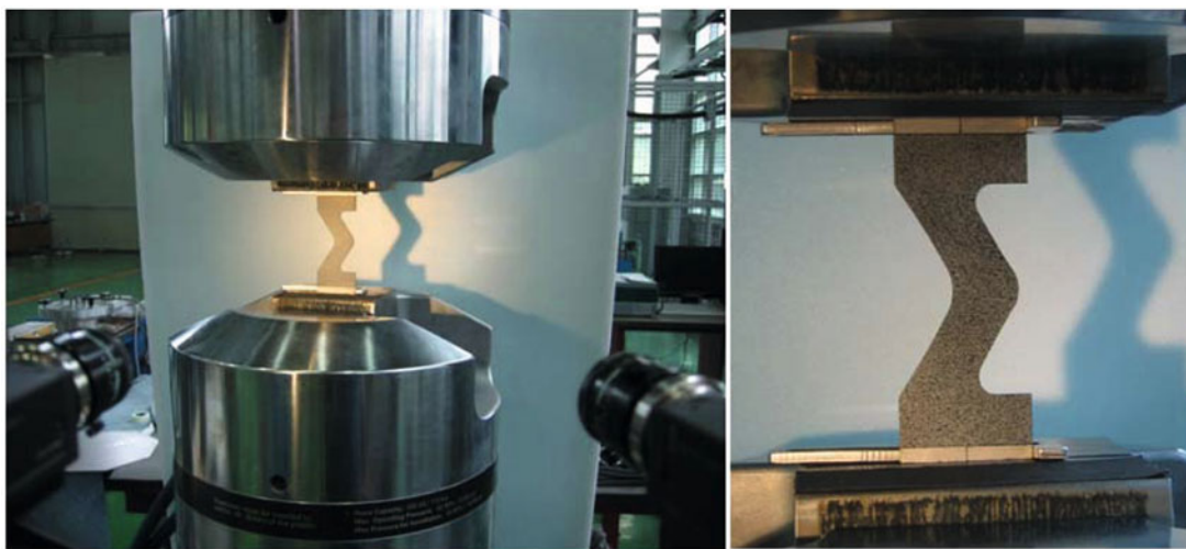
Fig. 31.1 Views of stereo image correlation set-up
