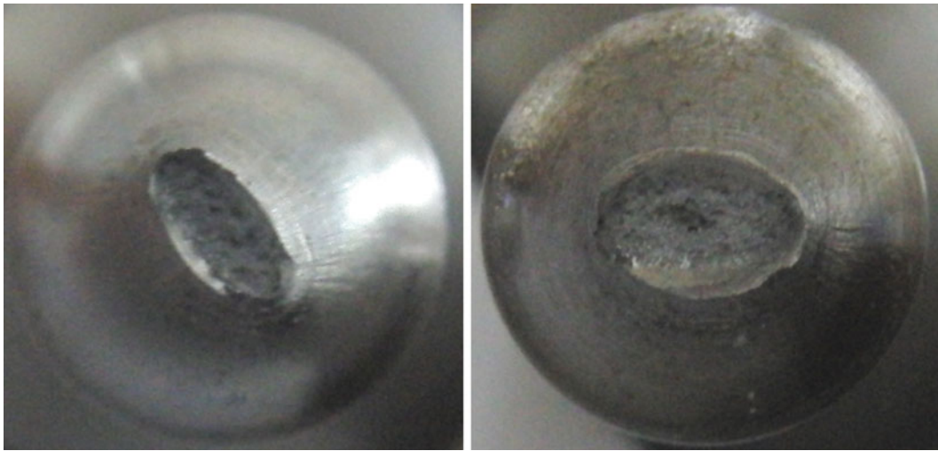
Fig. 33.7 Fractured notched tension specimens
