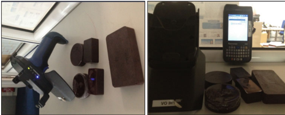
Fig. 21.7 Portable RFID chip reader to check the chip integrated in the composite samples
