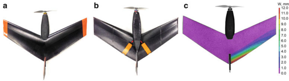
Fig. 12.3 (a) Top view of the forward swept wing aircraft, (b) bottom view of the aircraft with MFCs in view. (c) Out-of-plane deflection as measured by digital image correlation (DIC) when right MFC is actuated to 1,500 V
