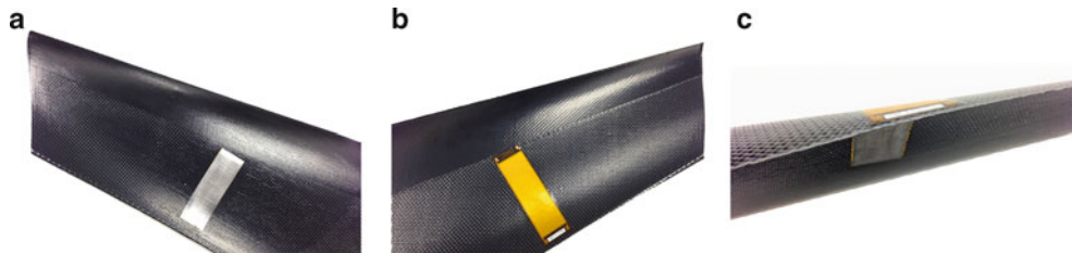
Fig. 12.18 (a) Top view of the steel embedded within the wing, (b) bottom view of the same wing, (c) rear view of the wing
