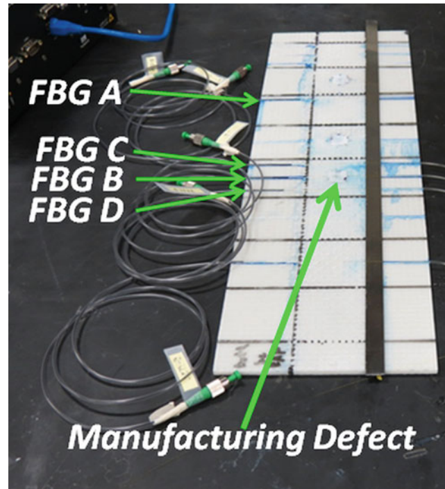
Fig. 22.2 Manufacturing of composite single-lap joints with embedded FBG sensors
