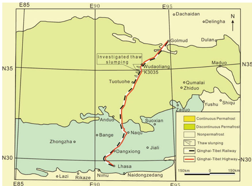
Fig. 1 Distribution of the permafrost and the thaw slumping on QTP
