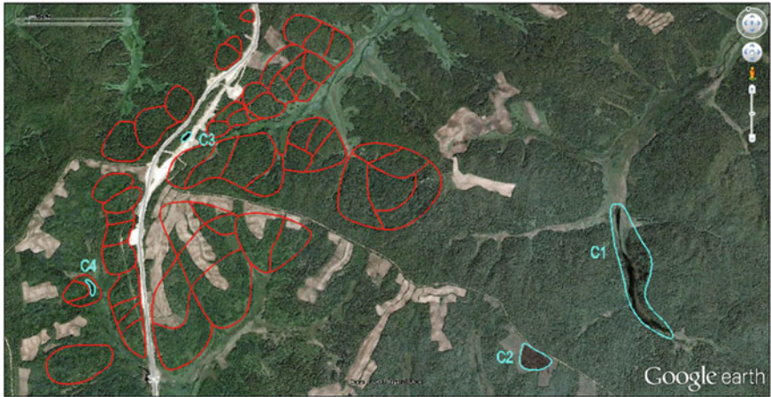
Fig. 5 Creeping platform and the distribution of melting permafrost in study area
