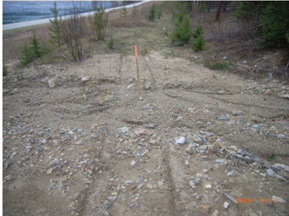
Fig. 7 Pre-season tire tracks over the landslide deposit. This likely happened when there was thin snow cover—sufficient to hide the deposit, but not enough to prevent impressions in the wet mud
