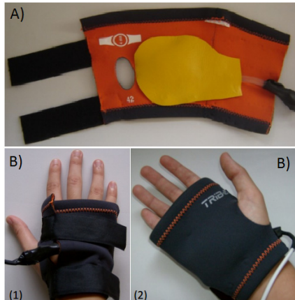
Fig. 1 Device developed by Inês Clemente [12] to assess muscular spasticity A) Inside view of “The Glove” (Small water bag inserted in between the glove tissue and the yellow cover tissue). B) Outside view of the Glove, (1) back of the hand (2) and palm view [12].
