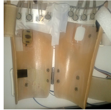
Fig. 4 Sensor arrangement in the prosthesis socket
