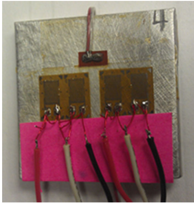
Fig. 48.9 Arrangement of four strain gages and type-J thermocouple on 1/8" (3 mm) thick aluminum block
