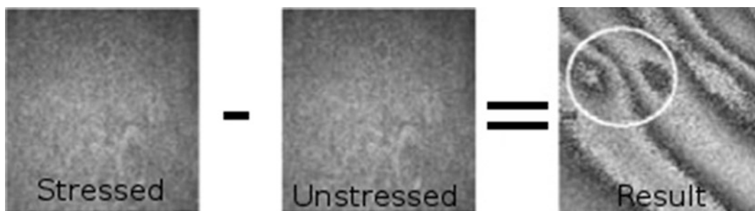
Fig. 34.2 Phase images of stressed and unstressed component and the resultant phase stepped fringe pattern
