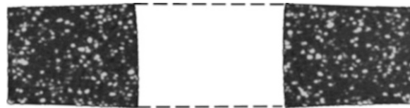
Fig. 27.2 Centerline cross-section of deformed specimen after applying compressive loading
