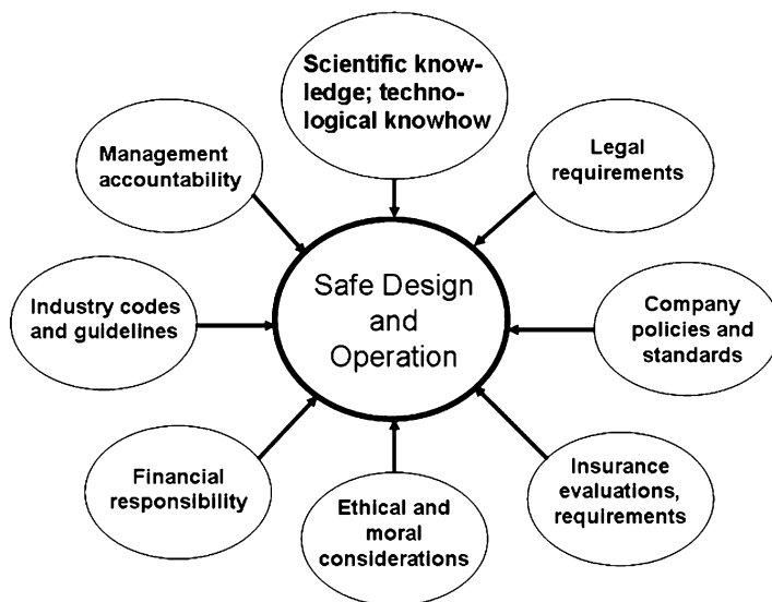
Fig. 4.19 Major factors determining safe chemical plant design and operation (Adapted from [26])
