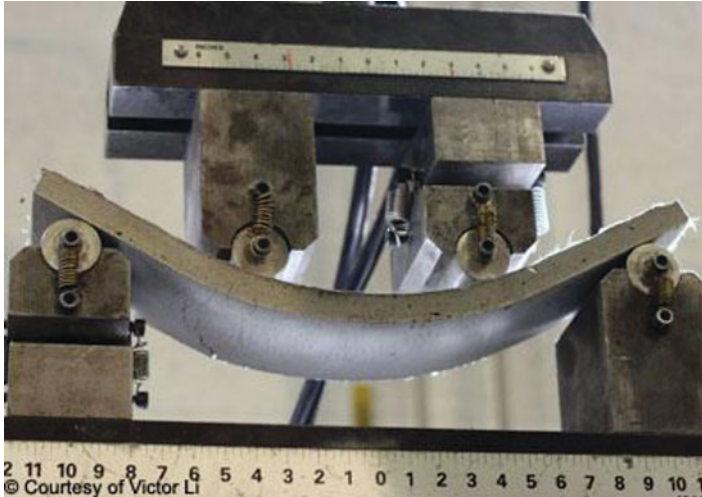
Fig. 7.32 ECC material in pure bending reveals large deformations due to multiple cracking [22] (Courtesy Prof. Li)
