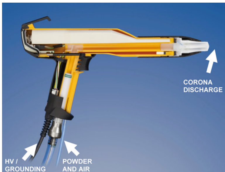
Fig. 13.3 Schematic representation of a conventional corona gun from ITW-GEMA. Corona discharge happens at the end of the electric filament running through the center of the spray nozzle (Reproduced with permission of GEMA GmbH)
