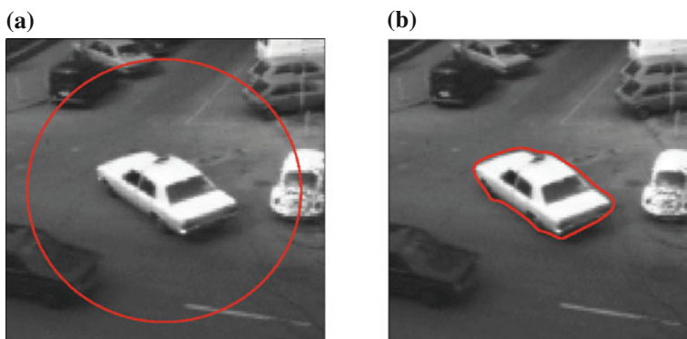
Fig. 1.3 Motion detection by minimizing a functional measuring the amount of optical flow contrast along a geodesic active curve: a The first of the two consecutive images used, and the initial curve superimposed and, b the final position of the curve. The active curve settled on the moving object boundary due to the strong image motion contrast along this boundary
