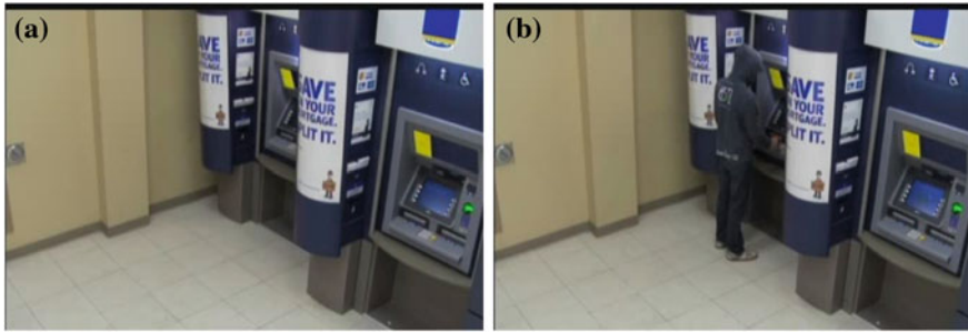
Fig. 4.6 Motion detection by background subtraction: a the template image of the scene; it contains only the objects that are normally part of the scene and are static during the detection process and, b an image of the current scene, in which motion detection is to be performed
