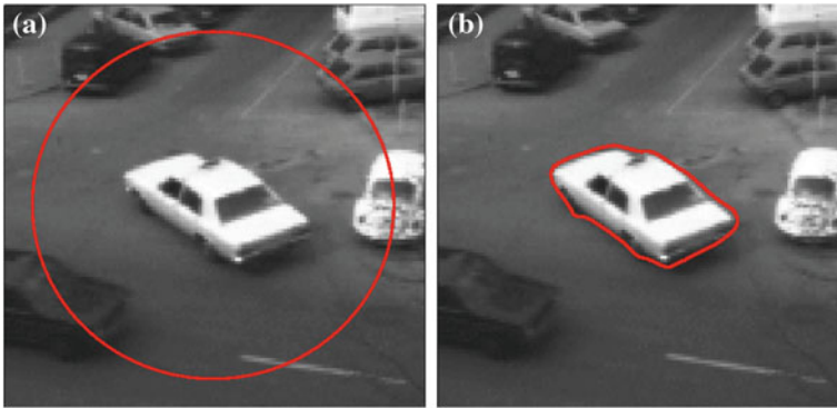
Fig. 4.15 Hamburg Taxi sequence: Optical flow based motion detection by minimizing the geodesic functional of Eq. (4.69) via the curve evolution equation (4.71). The white car proceeding through the intersection is the single moving object: a shows the image with the initial geodesic curve placed wide enough to contain the image of the moving car; b shows the motion boundary detected by the geodesic curve at convergence
