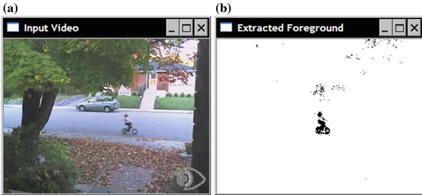
Fig. 4.3 Stauffer-Grimson motion detection method by mixture of Gaussians modelling of intensity: a The observed scene; everything is motionless in this scene except the tree foliage and the bike and its rider. b The detected foreground points. The points are on the image of the bicycle and its rider, and at the fringes of the tree foliage where the intensity variation between consecutive frames is more noticeable
