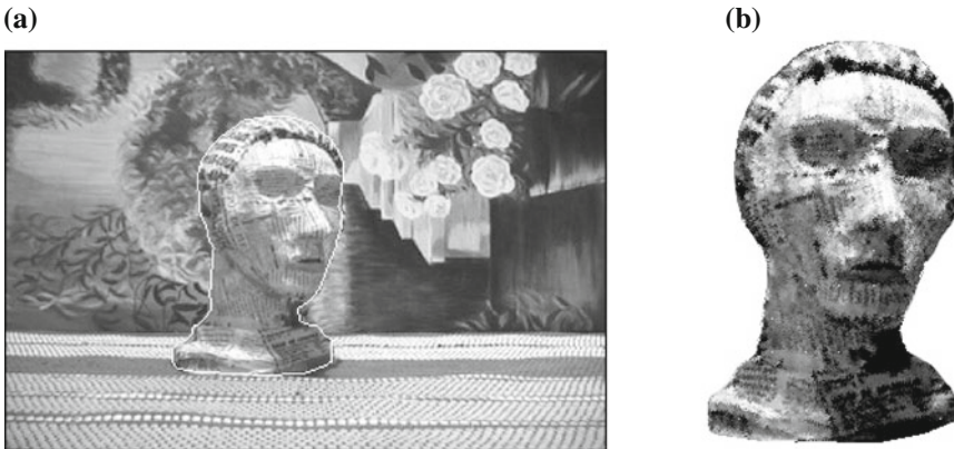
Fig. 1.5 Dense three-dimensional interpretation of optical flow by an active contour variational method [41]. The camera is static. The figurine moves in a static background. a The method was able to outline the moving figurine using 3D motion information which was concurrently recovered. b Displays a view, from a different angle, of the depth of the figurine constructed from the scheme's output
