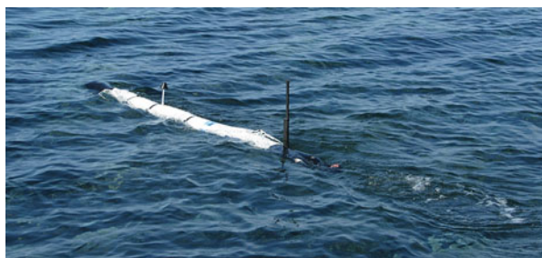
Fig. 2 AUV equipped with sensor system floating on seawater
