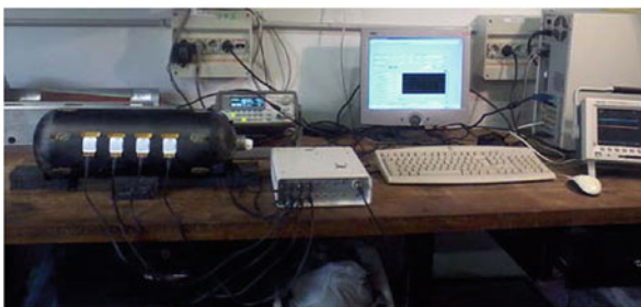
Fig. 3 Programmable acquisition system for active SHM on COPV with interdigital PPTs network
